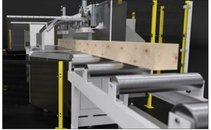
Handling solutions: customized roller tables and support planes.
